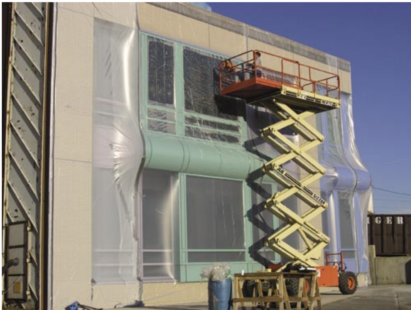
Laboratory mockup during an ASTM E283 air infiltration test, which tests assemblies of opaque walls, curtain walls and windows.
