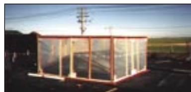
Figure 4: Chamber for pressurization/depressurization tests.
