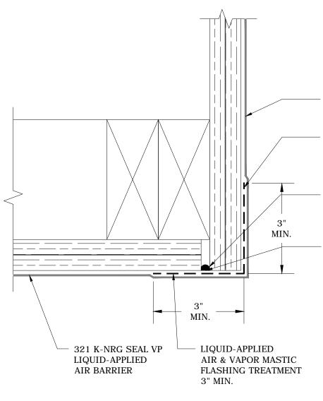
321 K-NRG SEAL VP LIQUID-APPLIED AIR BARRIER
