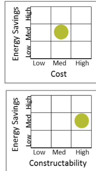
Figure 5: Cost and constructability analysis against energy savings for PIR foam board retrofit.
