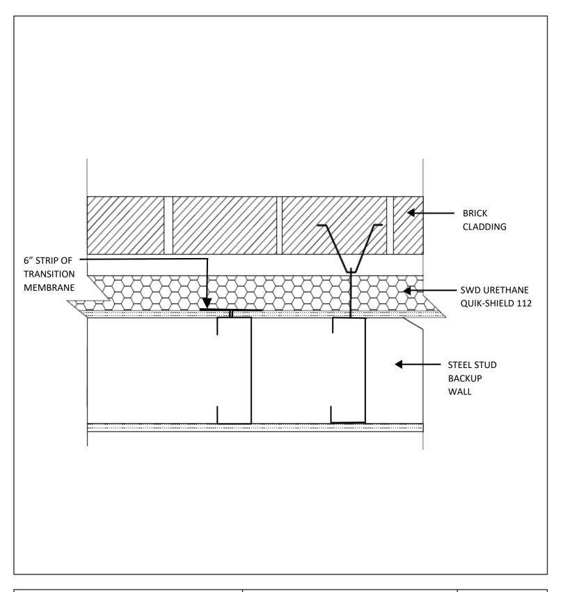
Sketch: STEEL STUD SUBSTRATE JOINT
