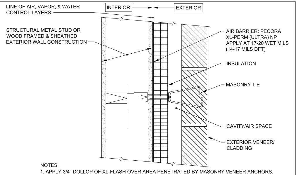
2. DOLLOP OF XL-FLASH IS NOT REQUIRED WHERE GASKETED MASONRY VENEER ANCHORS THAT SEAL TO CURED XL-PERM (ULTRA) NP ARE INSTALLED.
