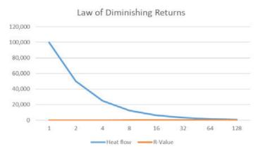
with R1 to R2, then R4, R8, R16, R32, R64, R12 progressively multiplies the slowing of heat flow.
