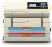
We test the materials at a mean temperature of  $75 \pm 2^{\circ}$  F ( $24 \pm 1^{\circ}$  C) with a temperature differential of  $40 \pm 2^{\circ}$  F ( $20 \pm 1^{\circ}$  C). At  $75^{\circ}$  F, we probably do not need any insulation. The purpose of this test though, is to allow a person to
