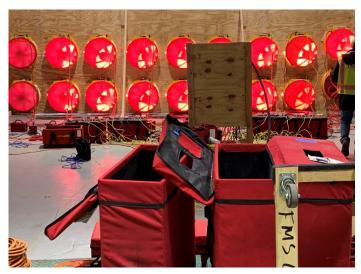
It turns out that we don't know yet. I witnessed a whole building blower door test on a 1,000,000 square foot building that occupied a whole city block in New York, NY. The building was twelve stories high with a footprint of around 90,000 square feet. The surface area of the six sides of the building was
