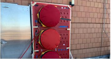
The two major items with this change are the target rate for air leakage (0.25 cfm/ft2) and that if the result exceeded 0.40 cfm/ft2, it needed to be rectified and re-tested. Anything above 0.40 cfm/ft2 would NOT be accepted.
