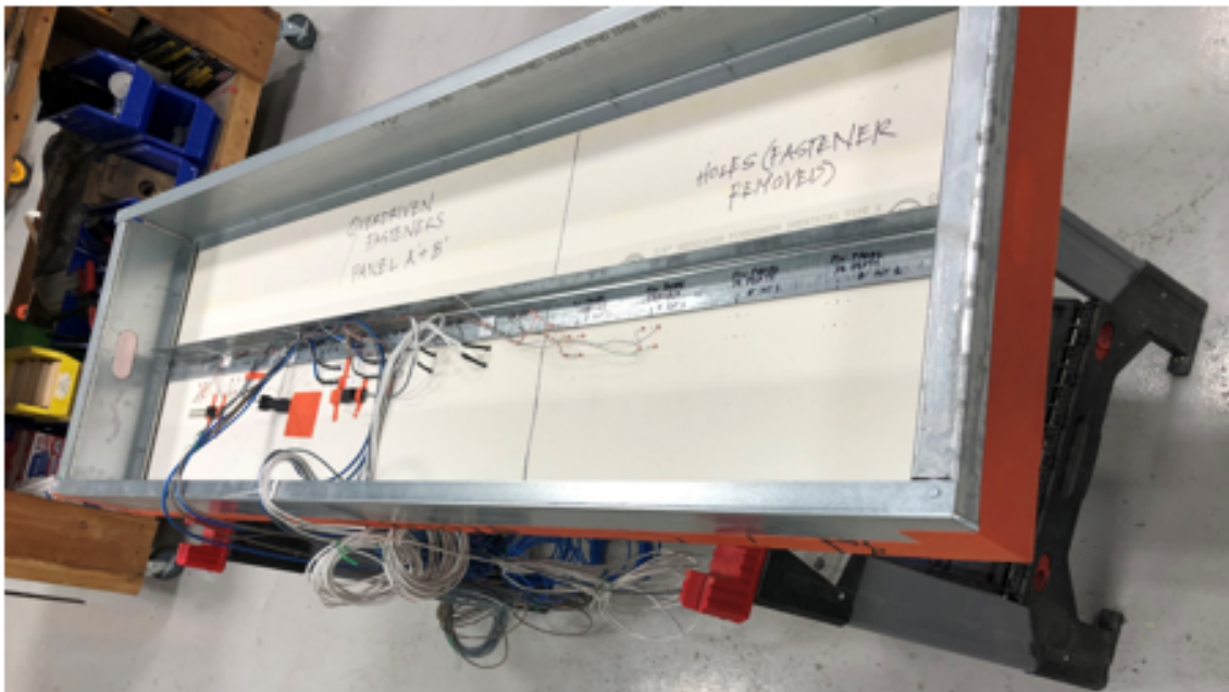
Figure 7: Test panel A/B during the application of the sensors.
