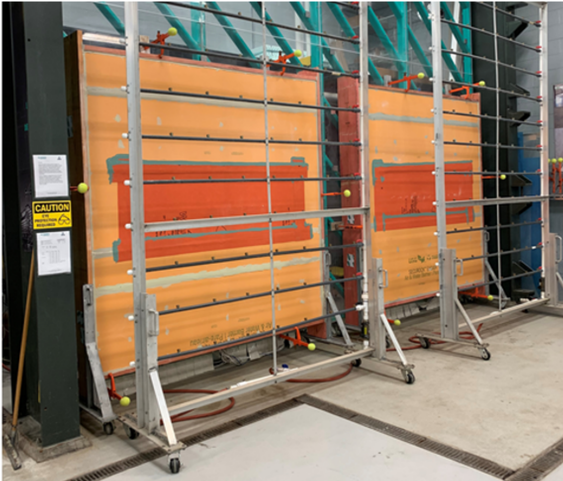
Figure 6: Test panels installed in an ASTM E331 apparatus.
