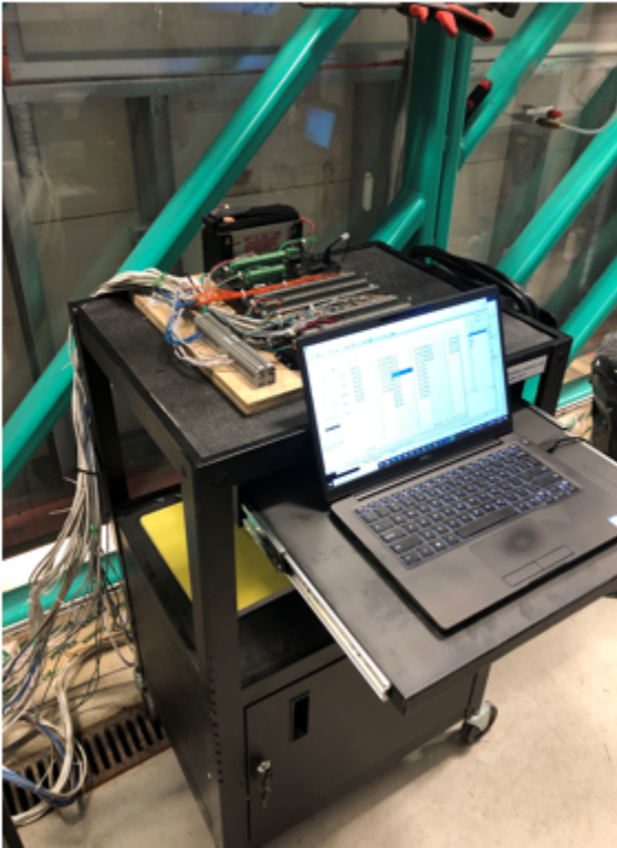
Figure 7: Data collection systems were used to collect and store data outputs from sensors installed in the test panels. Computers were connected to the data loggers (left photo) for this purpose. Campbell Scientific data loggers were used to collect real time data (right photo).
