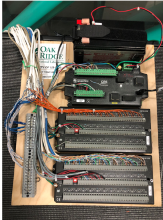
Figure 7: Data collection systems were used to collect and store data outputs from sensors installed in the test panels. Computers were connected to the data loggers (left photo) for this purpose. Campbell Scientific data loggers were used to collect real time data (right photo).
